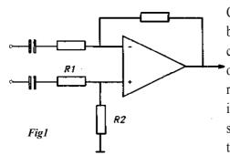
Circuits such as in Fig.l offer a little isolation from ground, but it is not sufficient isolation. This circuitry also has other characteristics that are undesirable: the input impedance on the non-inverting leg is permanently defined by the resistor value Rl and R2, while the input impedance on the inverting leg is changing dynamically with the signal. With signal the non-inverting input is of course moving and therefore the reference point for the inverting leg is changing.
