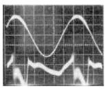
Fig.4: Sine Wave 1.6 kHz / 13V RMS / Load = 8 Ohms (HF oscillation of amplifier under test)
