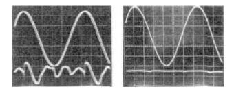
Fig. 1: Sine Wave 1.6 kHz / 40V RMS / Load = 4 Ohms
